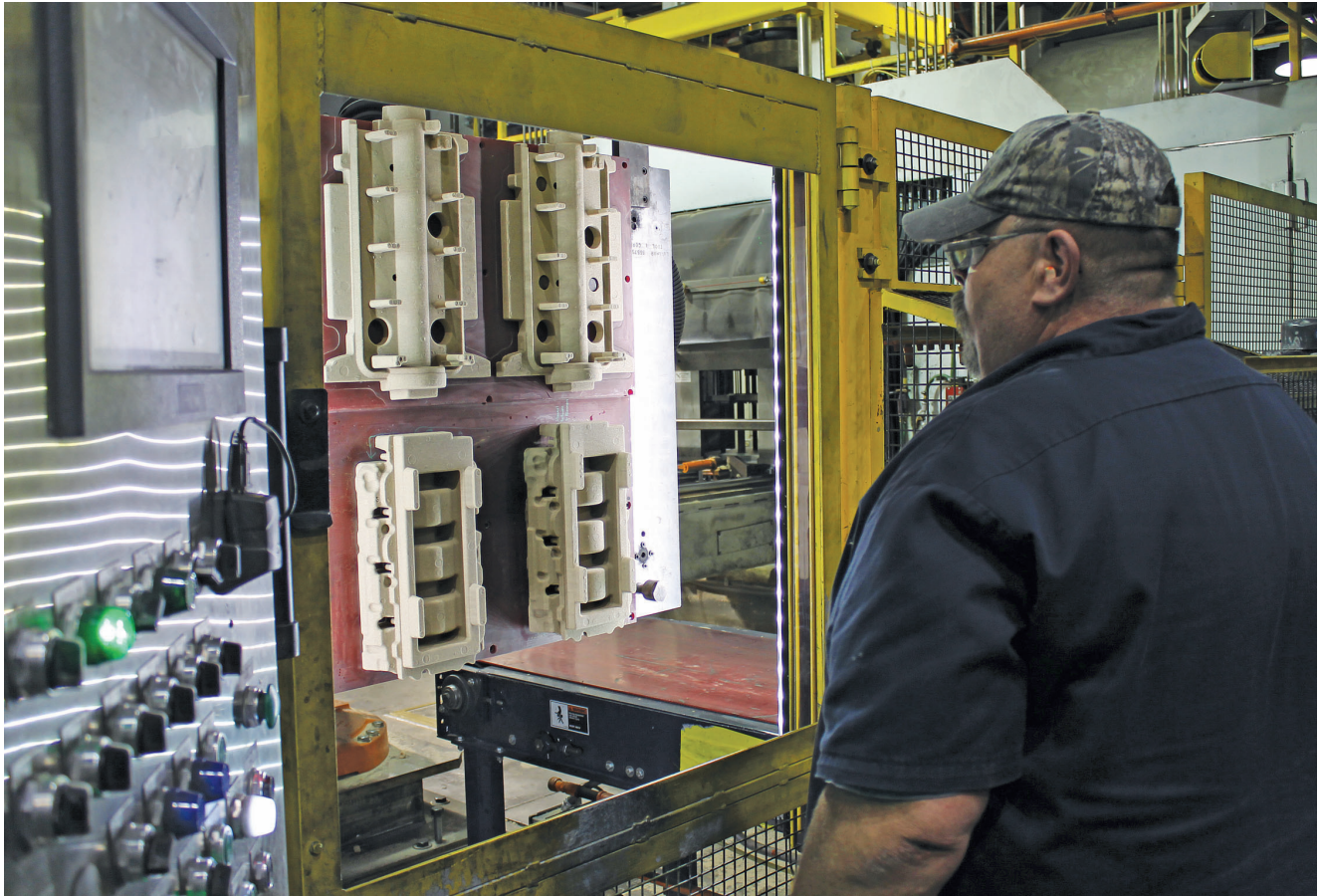
Two robotic cells produce the core assemblies for the hybrid car engine bedplate casting at Waupaca Foundry.
