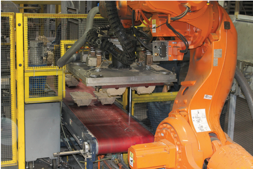
Reducing human touches on the core assemblies ensured the surface of the core would not be damaged, resulting in a superior casting surface finish.
