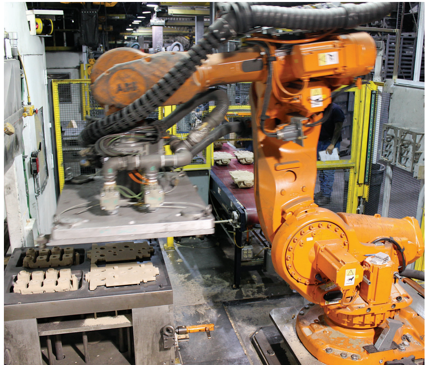
Robotic vacuum extractors handled the core assemblies throughout the process.
