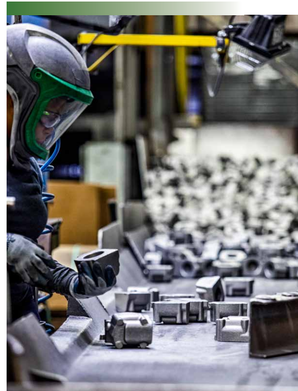
A mill room operator inspects gray iron castings on a finishing line conveyor to ensure they meet customer specification.
