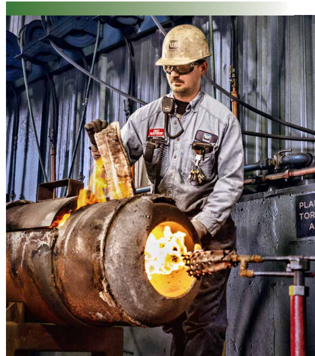
Melt foreman, William Mork lays a piece of refractory insulation to protect the furnace launder from high heat.
