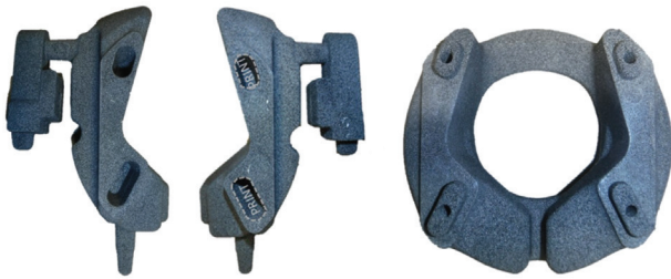
BEFORE: 3-Piece Cold Box Core
