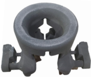
AFTER: 1-Piece Printed Core
