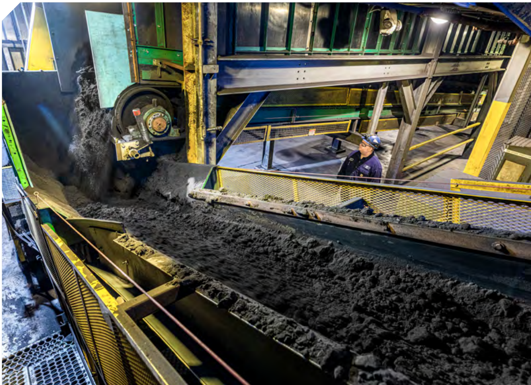
Recycled foundry sand is transported via conveyor and will be reused to make new sand molds in the iron casting production process.
